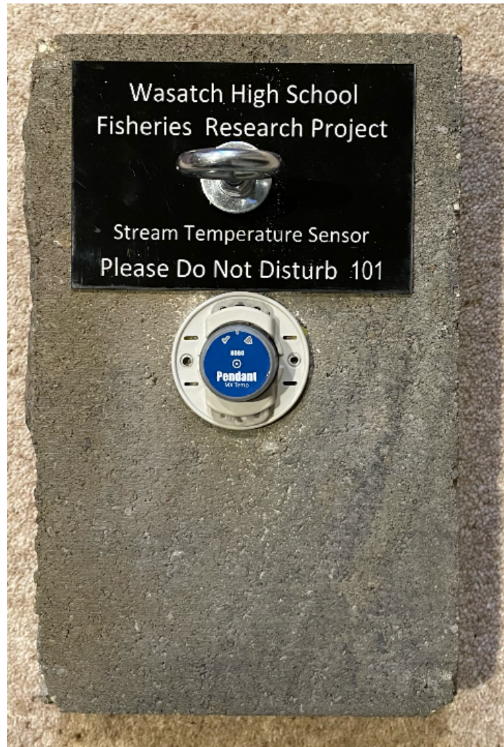
Figure 2. HOBOTemperature® temperature datalogger secured to a paver. The paver is inserted and removed from the water using a stick with a hook on the end that is inserted into the eyebolt. Once in the stream, the paver is soon covered by algae making it hard to distinguish from the rocks in the streambed.
